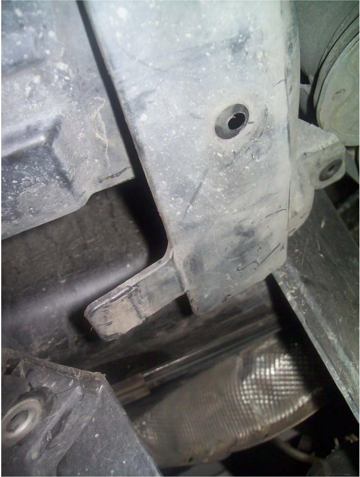
After wrestling with the cover and unclipping the emergency brake line that is attached at one of the corners, I was finally able to drop the cover onto the floor. I couldn't completely remove it so I twisted it a bit out of the way to make room to work on the filter.
