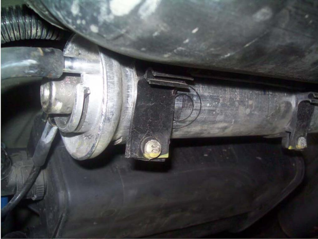
I oriented the filter with the vacuum line pointing to the front of the car. This makes it easier to connect all the lines back up.
