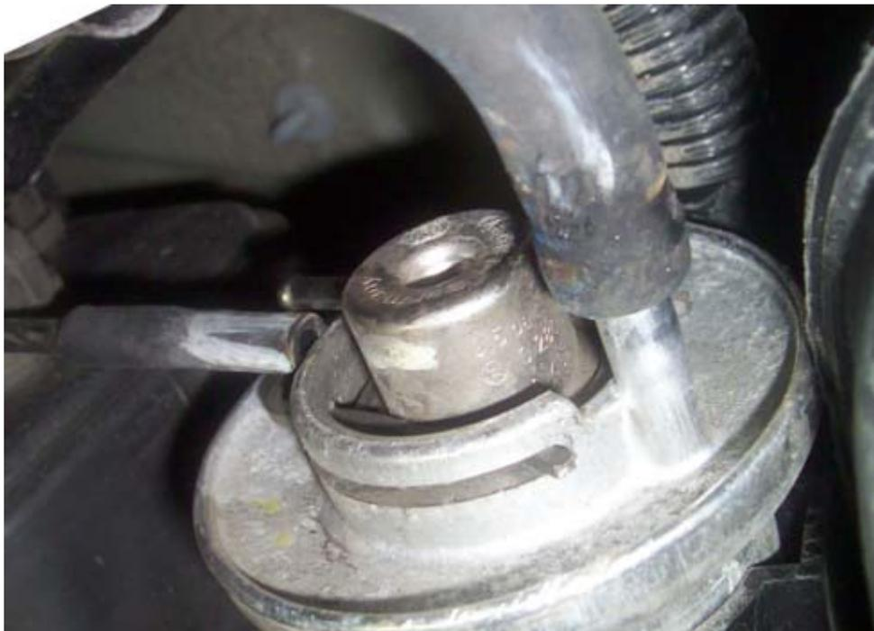
Next removed the crimped clamps on the opposite end of the old filter and connect them in the same locations one at a time on the new one.
