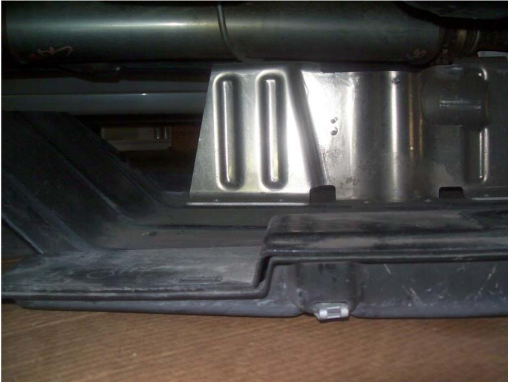
Note that the stamped flange you see reflecting is riveted to the gigantic plastic cover nearest the driveshaft. It takes some wiggling of the cover to get this flange to drop without removing the exhaust/driveshaft.
