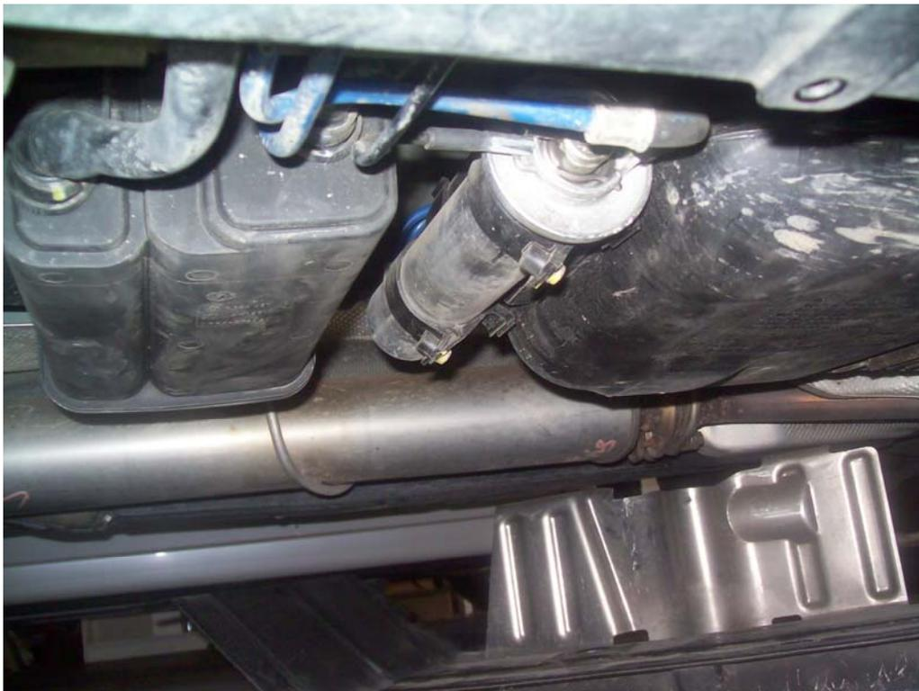
There is one outlet hose on the side with the pressure regulator and 2 inlets since I believe there are 2 fuel pump/sender units on the fuel tank. There is also a black plastic hose with a rubber end that connects to the vacuum line on the fuel pressure regulator (FPR). Here is a picture of the opposite end with the two fuel source input lines.
