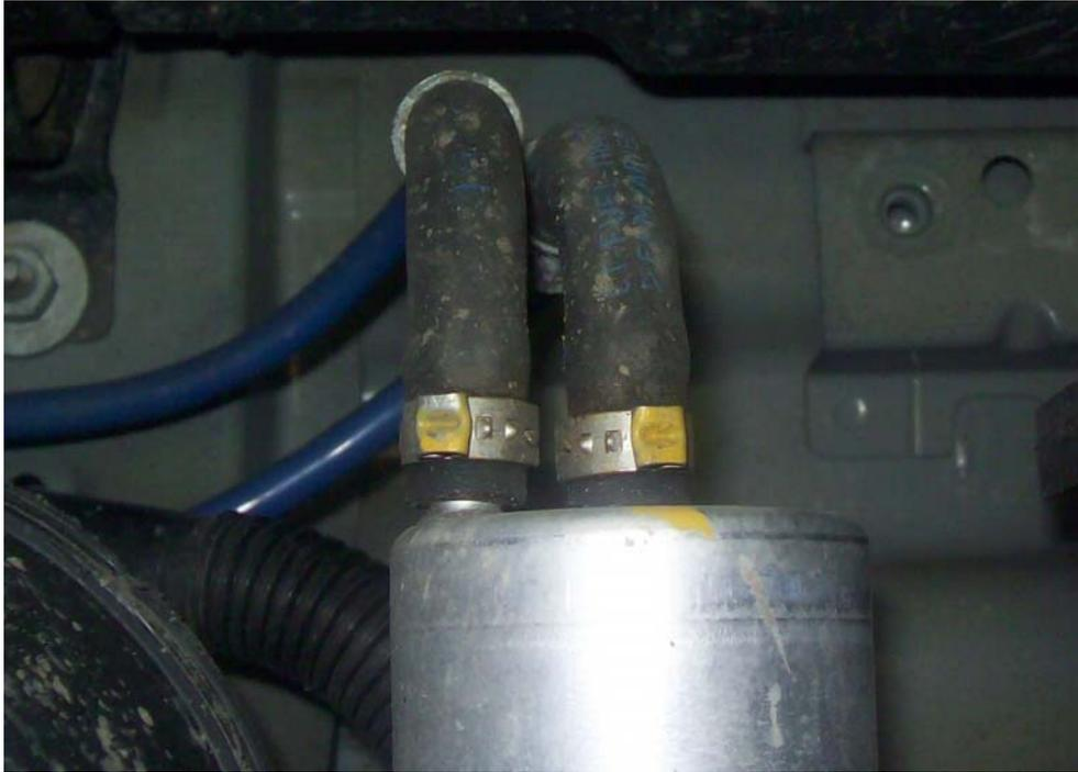
Next tighten all of the hose clamps and finally tighten the 2 screws holding the filter housing. Make sure you reconnected the vacuum line to the FPR. I then turned the key to the ON position without starting to pressurize the filter with fuel. I did this 3 or 4 times. I then started the car (of course after opening the garage door) and let it run for about 15 seconds. I then looked at the hose clamps to make sure I didn't have any fuel leaks.
