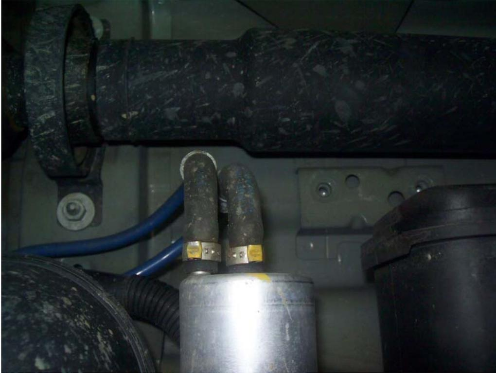
As you can see from the picture above, the fuel lines come from the factory with crimped clamps to hold the fuel lines in place. I used a pair of pliers to gently pry them open. I then used the tried and tested method of first twisting the lines to “break” the seal and then wiggling them off. If you simply try to pull them off, you run the risk of tearing them.
