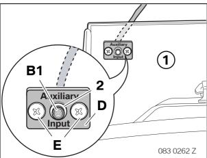
Insert branch **B1** in the glove compartment (1) and secure it to mounting plate **D** with a knurled nut (2).
