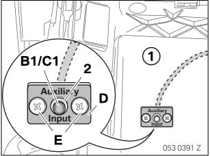
Insert branch **B1/C1** in the glove compartment (1) and secure it to mounting plate **D** with a knurled nut (2).
