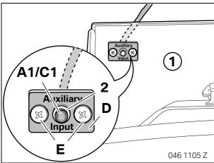
Insert branch **A1/C1** in the glove compartment (1) and secure it to mounting plate **D** with a knurled nut (2).
