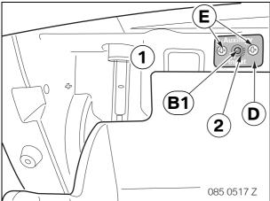
Insert branch **B1** in the glove compartment (1) and secure it to mounting plate **D** with a knurled nut (2).
