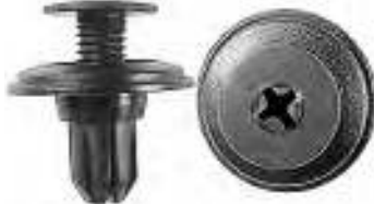
Art. # 150155197 Bumper & Fascia Attachments Push-Type Retainer NISSAN Hole: 11mm Head Dia.: 22mm Stem Length: 14mm Material: Black Nylon OE# 01553-03101
