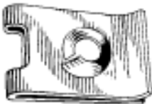
Art. # 150152086 "U" Type Nut BMW, MERCEDES, & VW Screw Size: 6.5mm Panel Range: .7mm-1.5mm CHE: 13mm Material: Plated MERCEDES-BENZ OE# 000-994-50-45 BMW OE# 0712-9-925-730 VW OE# N15.457.1
