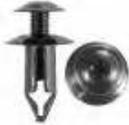
Art. # 150155581 Cowl Panel to Reinforcement Plate & Engine Splash Shield Ret. NISSAN, GEO Head Dia.: 14mm(9/16") Stem Length: 16mm (5/8") Fits into: 6mm (1/4") Hole Material: Black Nylon NISSAN OE# 66860-01W01 GEO OE# 94051993
