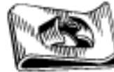
Art. # 150152082 "U" Type Nut BMW & MERCEDES Screw Size: 4.8mm Panel Range: .9mm-2mm CHE: 8mm Material: Zinc
