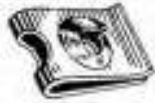
Art. # 150152083 "U" Type Nut VW Screw Size: 4.2mm (#8) Panel Range: .7mm-1.7mm CHE: 7mm Material: Plated OE# N15.422.2
