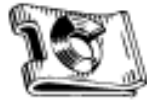
Art.# 150152084 "U" Type Nut BMW & MERCEDES Screw Size: 4.8mm Panel Range: .5mm - 1.7mm CHE*: 7mm Material: Plated BMW OE# 0712-9-925-737 MERCEDES OE# 000-994-06-45
