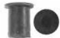
Art. # 150159537 Mirror/luggage rack Fastener Well Nut Head Dia.: .50" Length: .554 Hole: 3/8 Panel Thickness: .015-.150 Material: Neoprene w/ Captive Brass Nut
