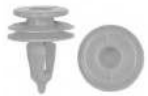
Art. # 150153195 Trim Panel Retainer CHRYSLER Top Head Dia.: 19/32" Bottom Head Dia.: 23/32" Stem Dia.: 5/8" Stem Length: 1/4" Material: Green Nylon OE# 6503204
