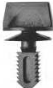
Art. # 150156077 Headlight Cover Retainer BMW Top Head Dia.: 15mm Bottom Head Dia.: 18mm Stem Length: 14mm Material: Nylon OE# 51711-916-197
