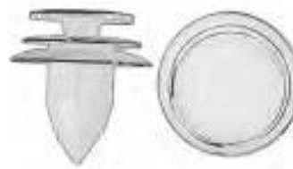
Art. # 150153197 Door Trim Panel Retainer CHRYSLER Top Head Dia.: 15mm Bottom Head Dia.: 20mm Stem Dia.: 9mm Stem Length: 15mm Material: Natural Nylon OE# 6505292AA
