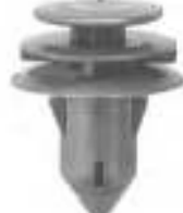
Art. # 150153548 Door Trim Panel Retainer CHRYSLER Head Dia.: Bottom: 20 mm Middle: 18 mm Top: 15 mm Stem Dia.: 9 mm Stem Length: 18mm Material: Gray & White Nylon
