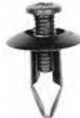
Art. # 150155574 Front Bumper Fascia Push-type Retainer NISSAN Head Dia.: 20mm Stem Length: 20mm Fits into: 8mm Hole Material: Black Nylon OE# 63854-01A00
