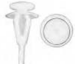
Art. # 150153207 Retainer-Door Cladding CHRYSLER Head Dia.: 12mm Hole: M7 Panel Range: 2mm Material: Nylon OE# MB566719
