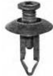
Art. # 150155704 Bumper Clip Push Type Retainer NISSAN Head Dia.: 20 mm Stem Length: 22 mm Fits into: 8 mm Material: Black Nylon OE# 63878-01E10
