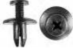
Art. # 150155586 Retainer NISSAN, HONDA, ISUZU Head Dia.: 15mm Stem Length: 11mm Fits into: 6mm Hole Material: Black Nylon NISSAN OE# 10998-30880 Isuzu OE# 8942981190 HONDA OE# 90684-SA5-0030
