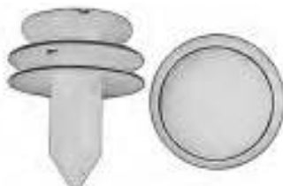
Art. # 150153209 Door Trim Panel Retainer BMW, CHRYSLER Top Head Dia.: 15mm Bottom Head Dia.: 18mm Stem Length: 14mm Stem Dia.: 8.5mm Material: White Nylon CHRYSLER OE# 6505539-AA
