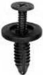
Art. # 150155401 Trim Panel Push-Type Retainer NISSAN Head Dia.: 11/16" Stem Length: 3/4" Fits into: 1/4" Hole Material: Black Nylon OE# N807578-S N808332-S
