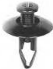
Art. # 150159543 Rivet-Screw Type Front & Rear Bumper Retainer NISSAN Head Dia.: 22mm Fits into: M8 Panel Range: 2-5mm Material: Nylon, Black High gloss Finish OE# 01553-02741, 01553-03201
