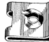
Art. # 150152081 "U" Type Nut MERCEDES-BENZ, BMW Screw Size: 4.8mm Panel Range: .8mm-1.7mm CHE: 11mm Material: Plated BMW OE# 0711-9-916-945 BENZ OE# 000-994-14-45
