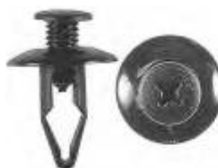
Art. # 150159598 Inner Retainer NISSAN Head Dia.: 20mm (25/32") Stem Length: 18mm (23/32") Fits into: 8mm (5/16") Hole Material: Black Nylon NISSAN OE# 63844-01A00 FORD OE# MNA01-56145 NA01-56145
