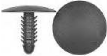
Art. # 150153141 Trim Panel Retainer CHRYSLER Top Head Dia.: 1/2" Bottom Head Dia.: 23/32" Stem Dia.: 5/16" Stem Length: 9/16" Material: Yellow Nylon OE# 6502907
