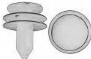
Art. # 150153209 Door Trim Panel Retainer CHRYSLER, BMW Top Head Dia.: 15mm Bottom Head Dia.: 18mm Stem Dia.: 8.5mm Stem Length: 14mm Material: White Nylon OE# 6505539-AA
