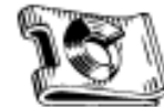
Art. # 150152084 "U" Type Nut MERCEDES-BENZ, BMW Screw Size: 4.8mm Panel Range: .5mm-1.7mm CHE: 7mm Material: Plated BMW OE# 0712-9-925-737 BENZ OE# 000-994-06-45
