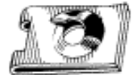
Art. # 150152091 "U" Type Nut BMW Screw Size: 5.6mm Panel Range: 1.2mm-2.0mm CHE: 10mm Material: Plated OE# 0712-9-925-720
