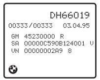
Note: As of 9/98 production the ZCS label was eliminated from the vehicle. Some older vehicles will have identification labels containing an AM segment, this information is not needed for coding or recoding a control module on that vehicle.
