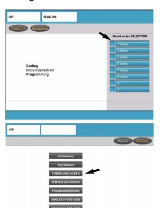
From Progman establish a connection to the interface connected to the vehicle and access CIP.
