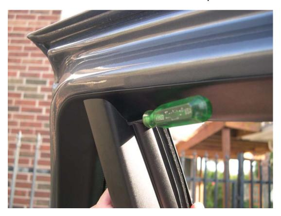
Next remove the T-20 Torx screw from the pillar
