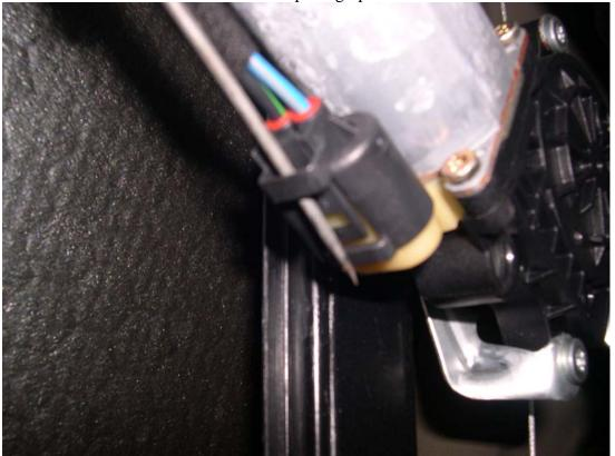
To remove the window regulator assembly maneuver it counter-clockwise to a 45 degree angle and slide it
