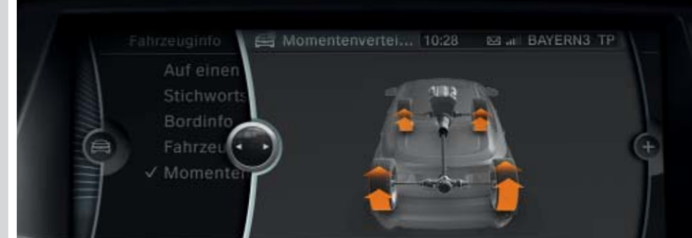
New: for the first time, the Control Display shows exactly, and in real-time, how xDrive and Dynamic Performance Control are splitting the drive power.
