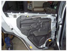
Step Five-Peel the black cover off using a sharp utility knife.
